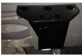
REMOVE EXISTING SCREW FROM BOTTOM OF DASH & DRILL 9/32 DIA HOLE FOR 1/4 x 1 BOLT & NUT
